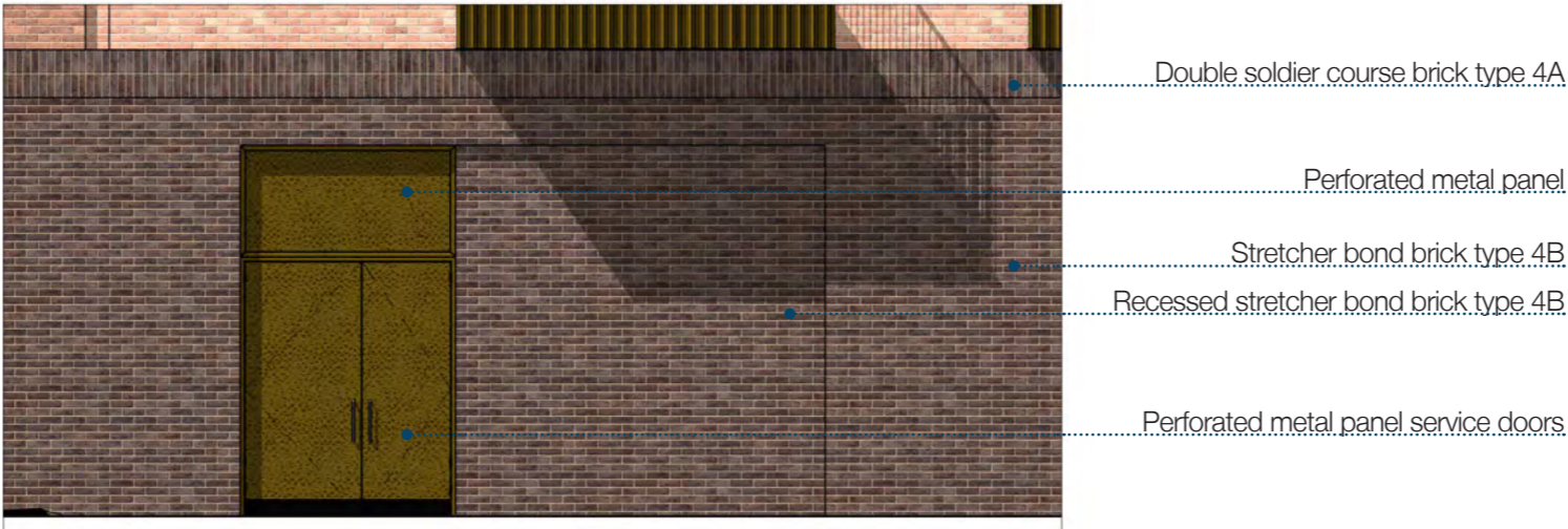
Figure 6.34: Detailed elevation study: refuse door
