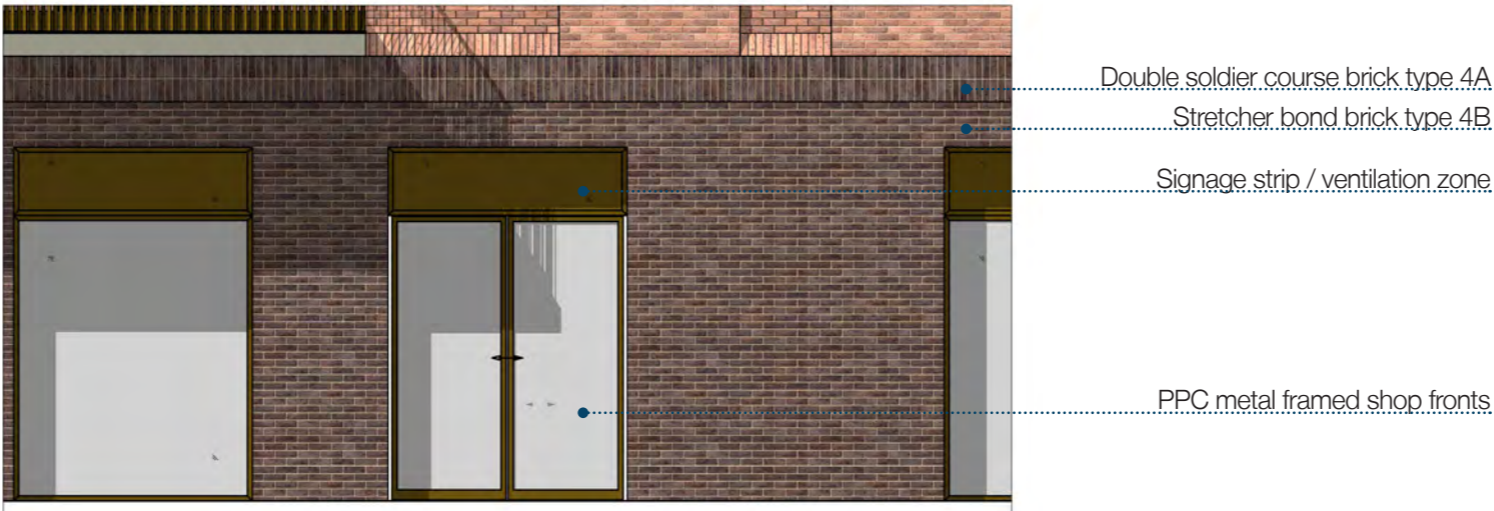
Figure 6.35: Detailed elevation study: shopfront and commercial entrance
