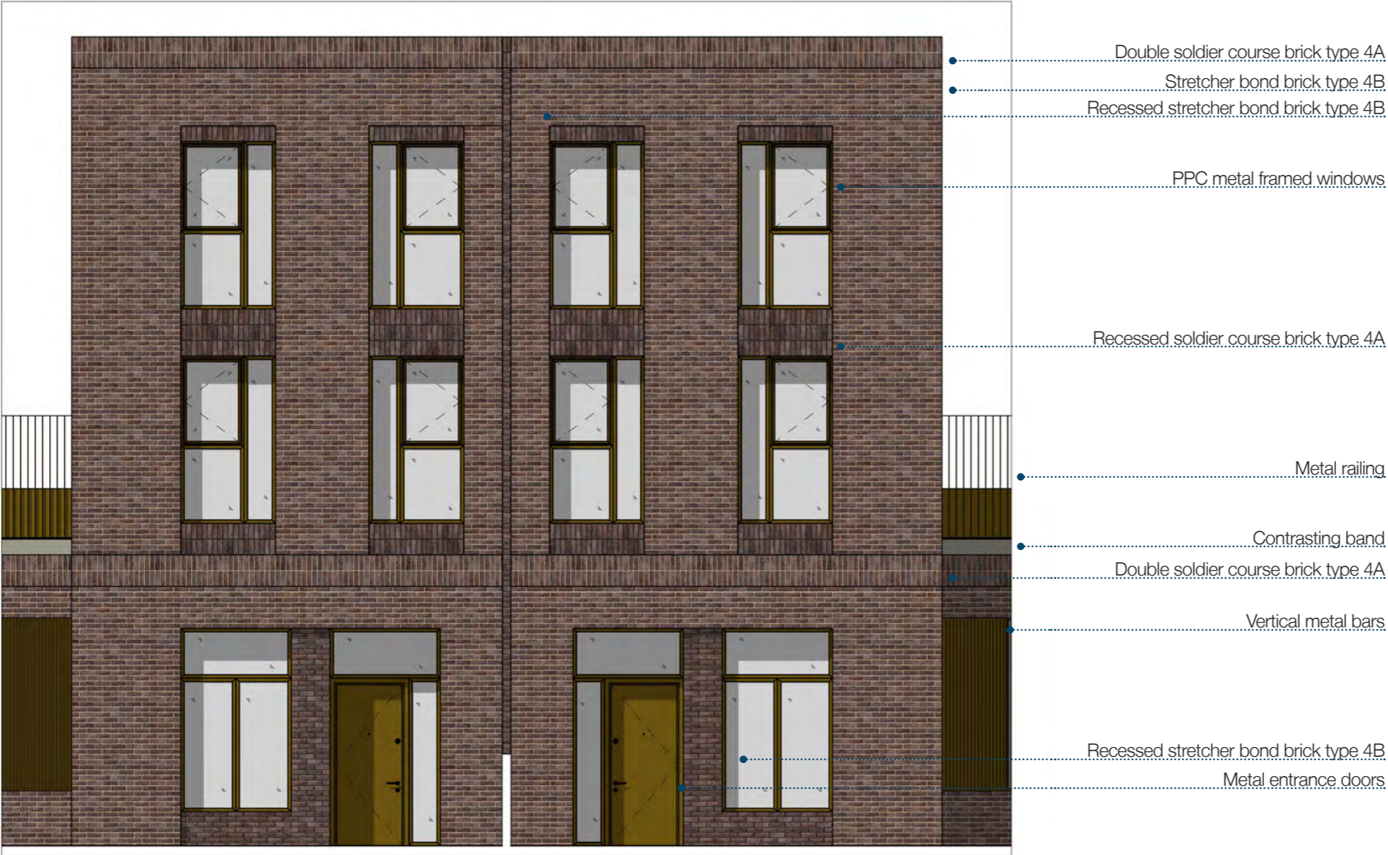
Figure 6.48: Detailed elevation study: houses
