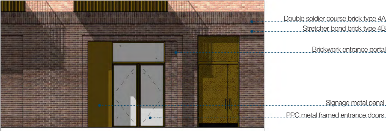
Figure 6.38: Detailed elevation study: communal entrance
