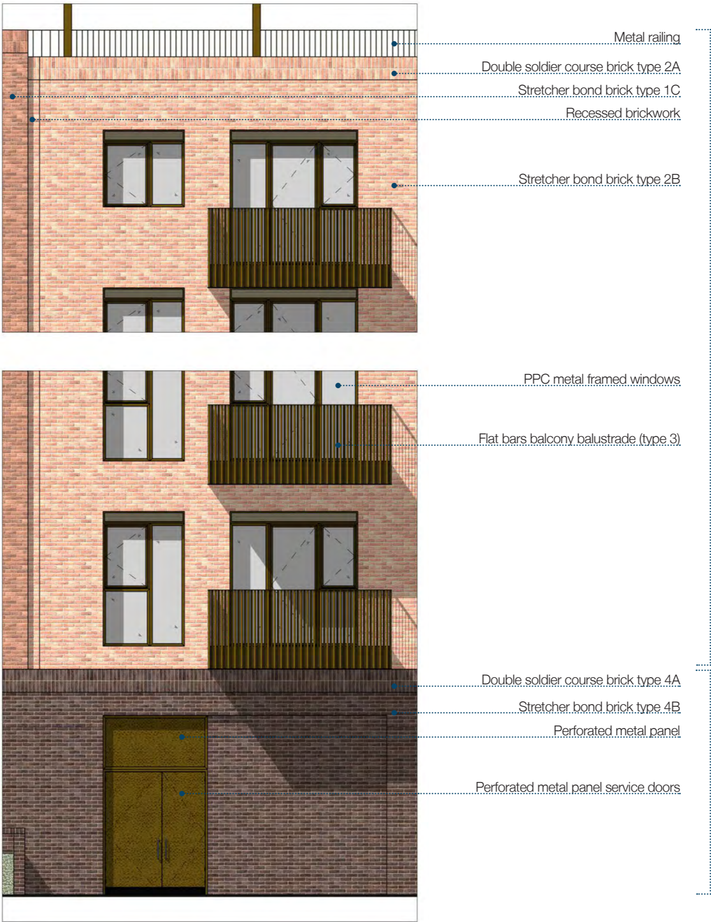
Figure 6.76: Detailed elevation study: street infill
