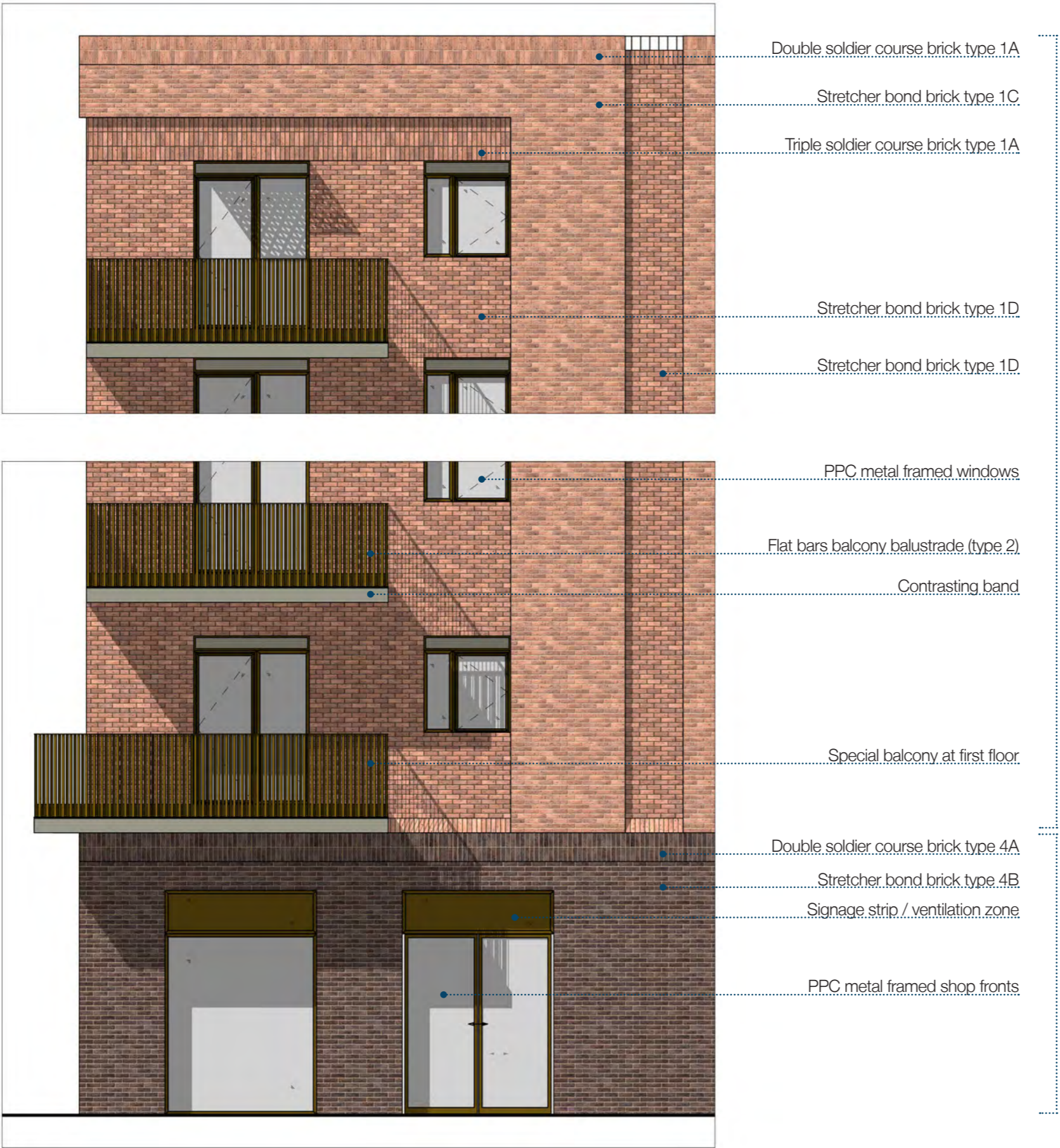
Figure 6.67: Detailed elevation study: bookend (A1 south facade)
