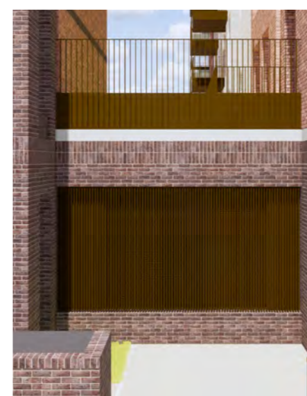
Figure 6.97: Ground floor ventilation panels
