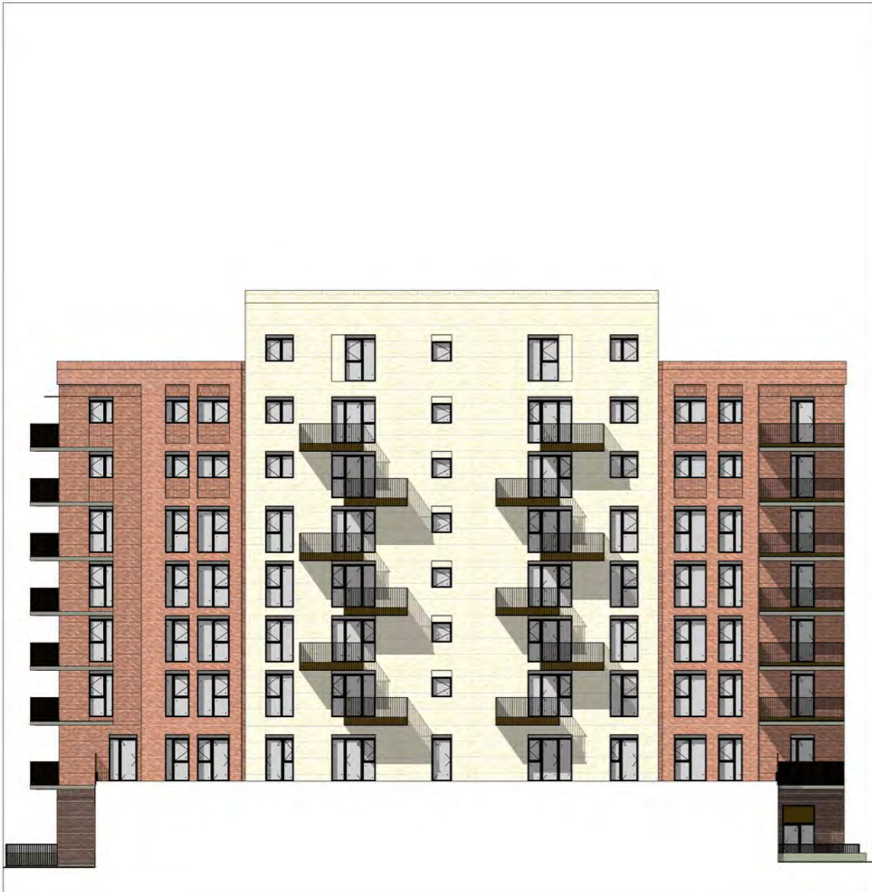
Figure 6.103: Proposed courtyard elevation: A1 east
