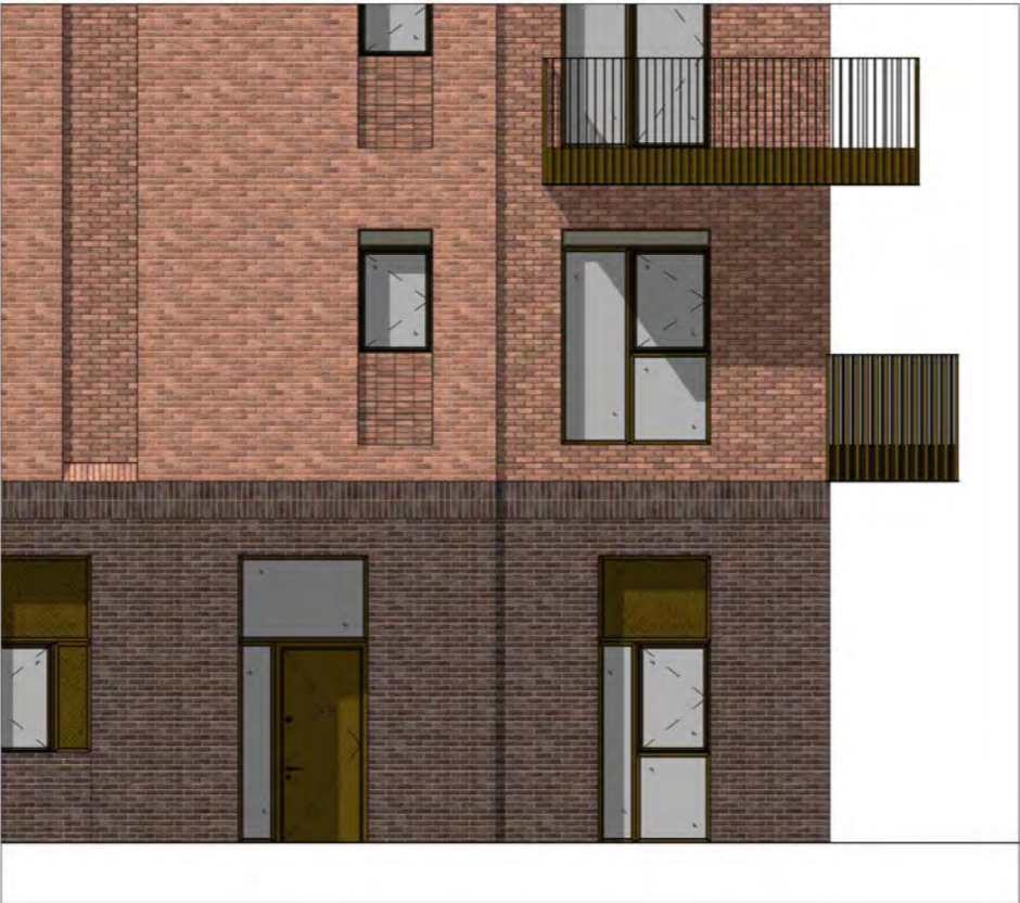
Figure 6.74: Detailed elevation study: bookend (A1 north facade)
