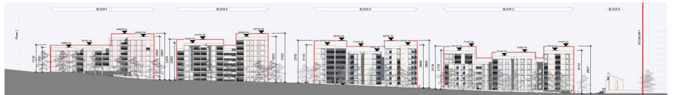
Building Elevations of consented scheme (Buildings C, D, E & F) with Red line depicting proposed increase to overall building height
