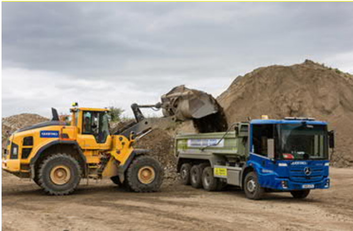
Figure 6-3 Example 32-Tonne Tipper Lorry
