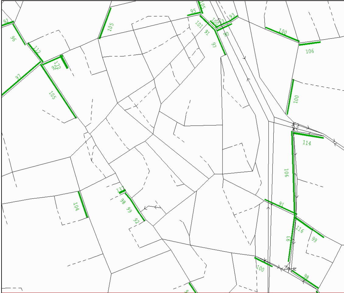
Figure A 14: DS 2021 (with Montrose and Peel Link) PM – V/C ratio bandwidth plot
