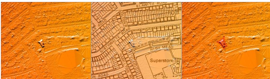
**Figure C-6 Poorly filtered buildings in Group 2 LiDAR**
